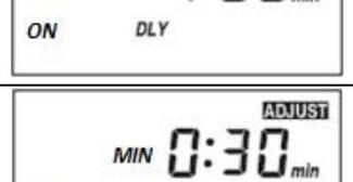
The display shows "ON" and "DLY" on the left. A large "1:00" is in the center with a small "min" to its right. A small "ADJUST" button icon is in the top right corner.  | On Delay                  | Interstage delay to activate the next stage                                                                                                                                                 | 0:10 to 8:00 minutes<br>Default = 1:00 minute              |
