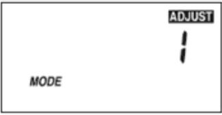
The display shows the word "MODE" on the left and a large digit "1" in the center. A small "ADJUST" button icon is in the top right corner.                                | Mode                      | Operating mode for the boiler.<br><b>NOTE:</b> A complete description of each mode can be found in section 8.4 Modes of Operation in this manual.                                           | 1 to 8<br>Default = 1                                      |
