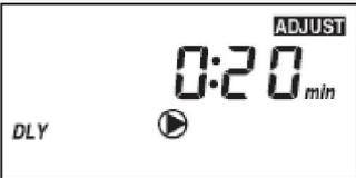
The display shows "DLY" at the bottom left, a large "0:20" in the center, and "min" at the bottom right. "ADJUST" is in a small box at the top right.                    | Pump Delay        | Boiler post pump time after burner has shut off, in seconds.                                                                                      | OFF, 0:20 to 9:55 min, On<br><br>Default = 1:00 min            |
