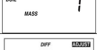
The display shows "BOIL" and "MASS" on the left. A large digit "1" is in the center. A small "ADJUST" button icon is in the top right corner.                             | Boil Mass (Mode 2 ONLY)   | Thermal mass of boiler. This determines interstage delay and minimum on and minimum off times.                                                                                              | 1 to 3<br>Default = 1                                      |
