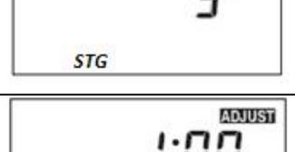
The display shows "DIFF" and "STG" on the left. A large "3" is in the center with a small "°F" to its right. A small "ADJUST" button icon is in the top right corner.    | Stage Differential        | Dictates the staging of the boiler and each stage is iterative. For example, if the value is 3°F. Stage 1 will be active 3°F below setpoint, Stage 1 & 2 will be active 6°F below setpoint. | Au, 2 to 42°F<br>(Au, -17 to 6°C)<br>Default = 10°F        |
