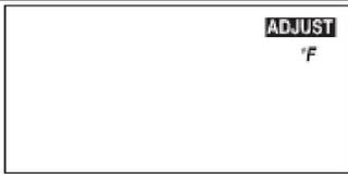
The display shows "ADJUST" in a small box at the top right and "°F" in the center.                                                                                      | Temperature Units | Select the desired unit of measurement                                                                                                            | °F, °C<br><br>Default = °F                                     |
